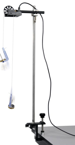
Figure 4: Setup for the Atwoods machine; you will start with 110 grams of added mass on each hanger and be able to take data for many mass differences. This apparatus was tested with mass differences of 2, 4, 6, 8, 10, 12, 14, 16, 18, 20, 22, 24, and 26 grams. Masses are transferred from mass 1 to mass 2.
